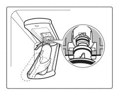
Rotate the water filter up into position and close the cover.
